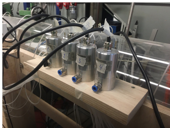
Figure 11. Differential pressure transducers used on the Venturi tube constriction section.
