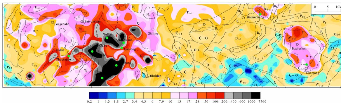
**Figure 6.** Sn geochemical map in the Gejiu area based on the fixed-value method. Color information is shown in Table 3. The geological legends are the same as those illustrated in Figure 1.
