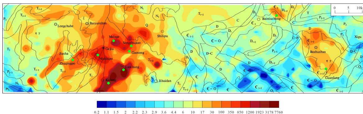
**Figure 3.** Sn geochemical map in the Gejiu area contoured using the cumulative frequency method. Color information is shown in Table 2 and geological legends are the same as those illustrated in Figure 1.
