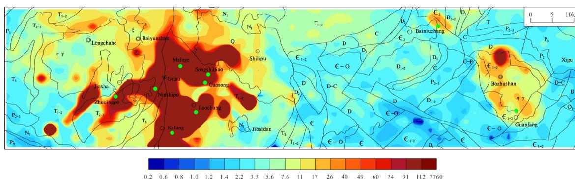
**Figure 5.** Sn geochemical map in the Gejiu area contoured using the  $Avg \pm k \cdot Std$  method. Color information is shown in Table 2. Geological legends are the same as those illustrated in Figure 1.
