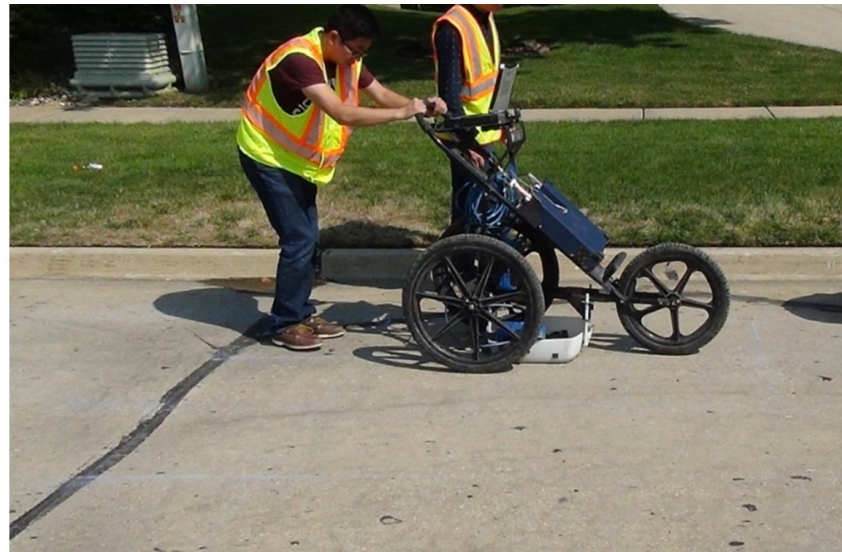
Figure 3. GPR survey conducted on a test site.
