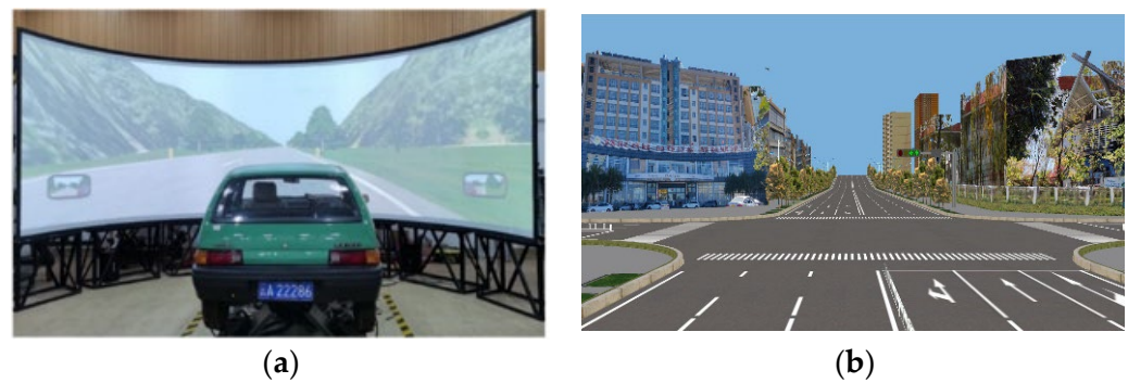
Figure 1. Experimental equipment. (a) KMRTDS driving simulation platform. (b) Simulated scenario.
