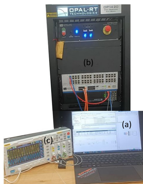
Figure 11. Real-time digital simulation setup for SST model validation. SST model has been developed using RT Lab (a), synchronized through the OPAL-RT simulator (b), and the output can be observed on an oscilloscope (c).
