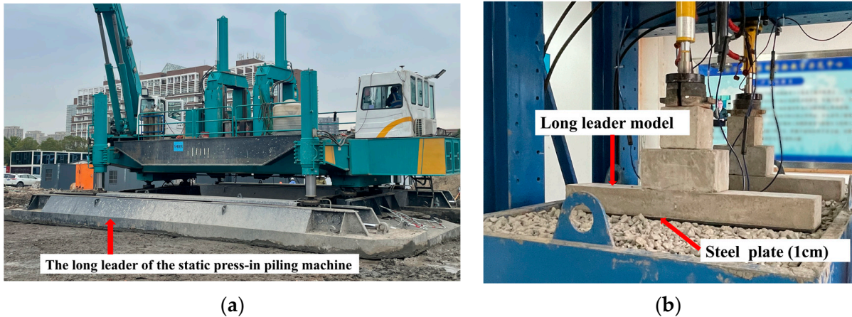
Figure 2. Schematic diagram of long leader for piling machine. (a) Piling machine in practical engineering. (b) Piling machine in model test.
