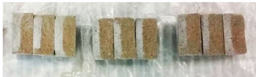
Figure 8. White silver precipitation of chloride salt.
