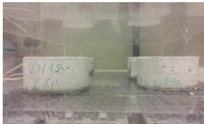
Figure 6. Water absorption by capillarity conducted in a water bath with an automatically adjusted water level.
