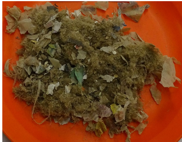
Figure 1. WG contaminants retained in the laboratory via a 1 mm sieve.
