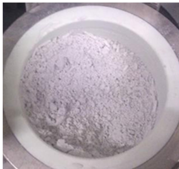
Figure 2. WG passed through a 1 mm sieve.
