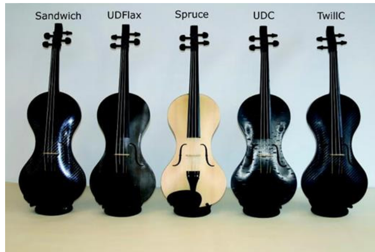
Figure 5. Prototype violins with soundboards from 5 different materials. Reprinted with permission from [12]. Copyright 2020, Acoustical Society of America.
