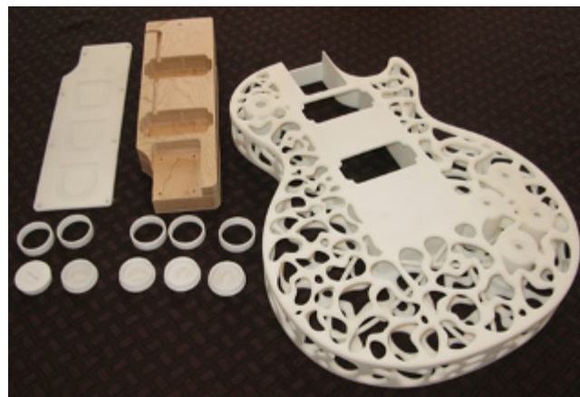
Figure 13. Final design of an ODD Guitar body using an internal wooden core. Used with permission of [Emerald Publishing Limited], from [5]; permission conveyed through Copyright Clearance Center, Inc.
