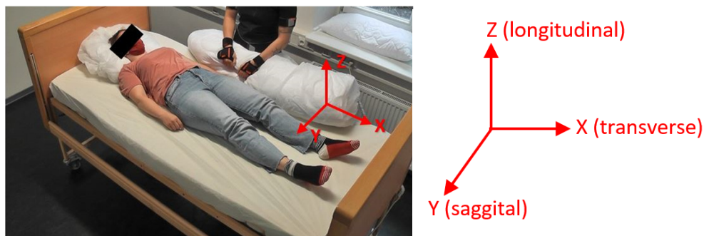
Figure 2. Xsens sensor coordinates placed on nurses' hands.
