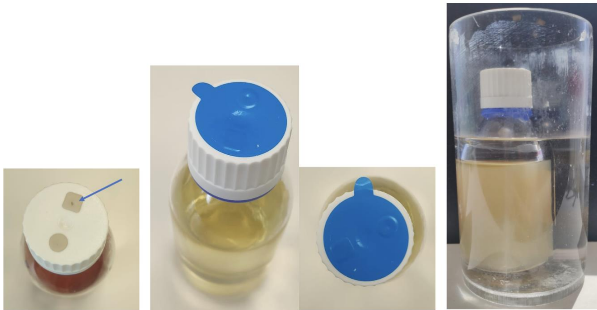
Figure 1. Design of the cap on the bottle for sterilization of culture media in a microwave oven equipped with a water bath.
