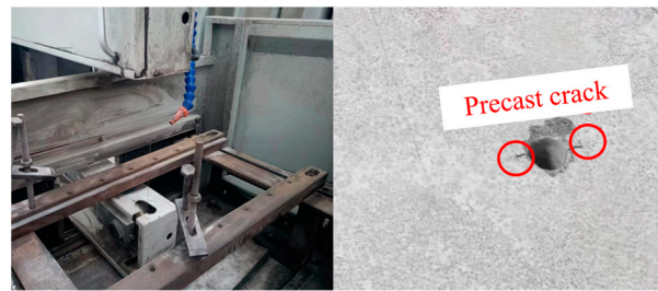
Figure 10. Precast crack making.
