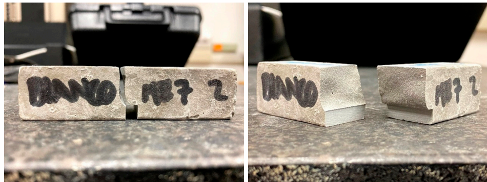
Figure 9. Linear crack path and smooth fracture surface. Plain cement (OPC) at 7 days.
