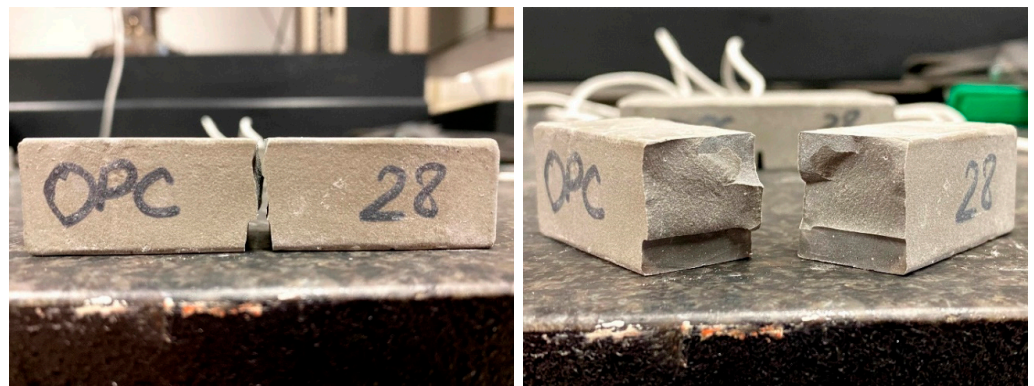
Figure 11. Linear crack path and pseudo-smooth fracture surface. Plain cement (OPC) at 28 days.
