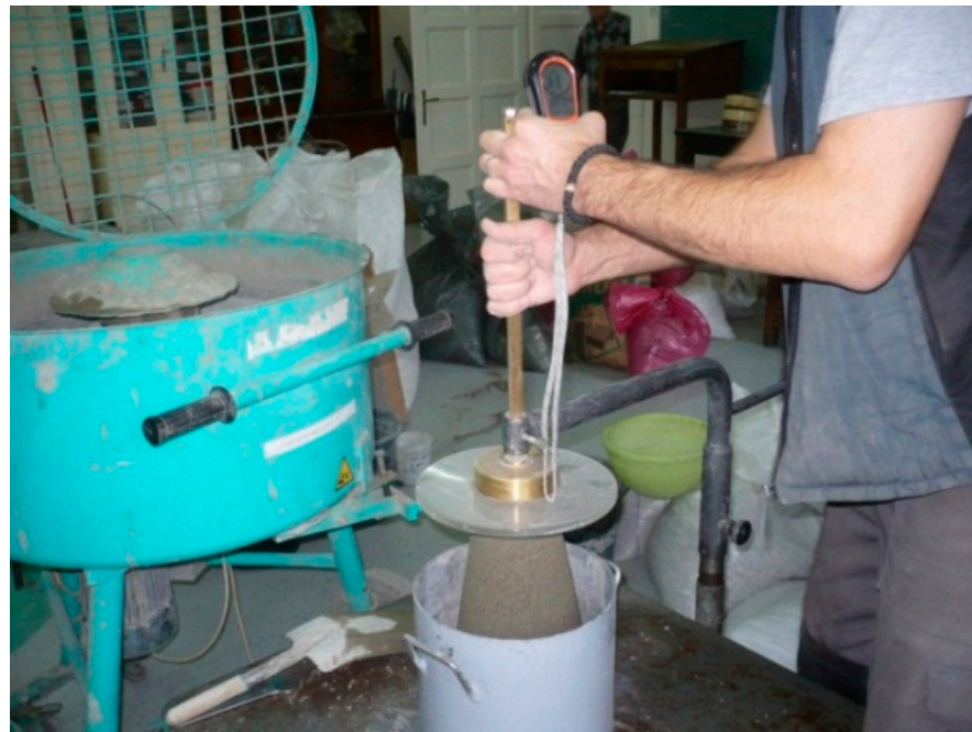
Figure 1. The procedure for testing consistency.
