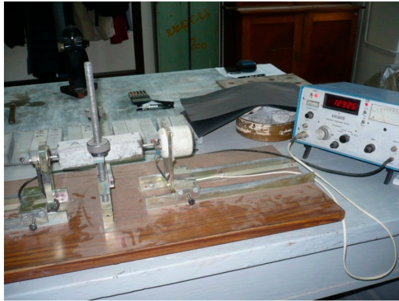
Figure 4. Disposition for testing the dynamic modulus of elasticity.
