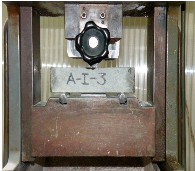
Figure 3. Testing the flexural strength on samples.
