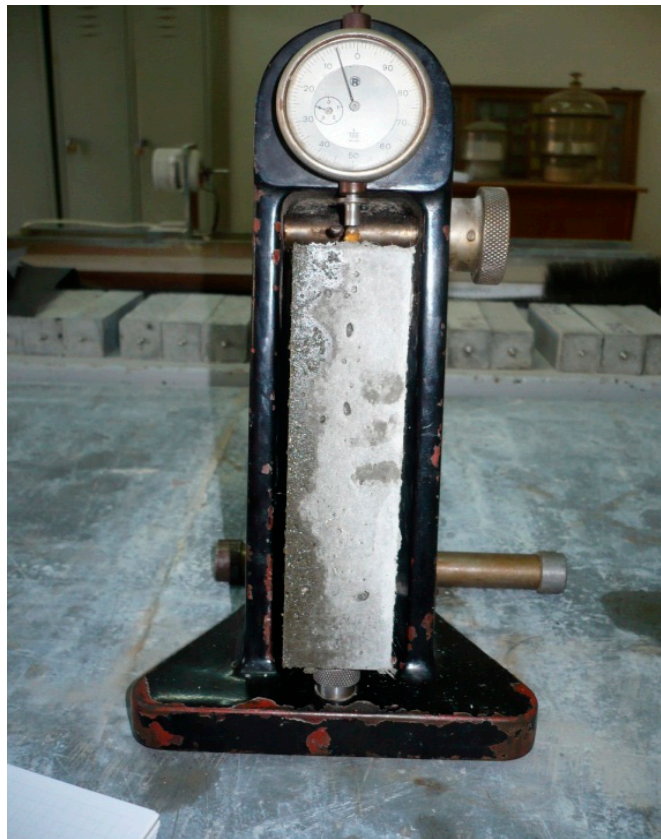
Figure 5. Shrinkage-deformation measurement comparator.
