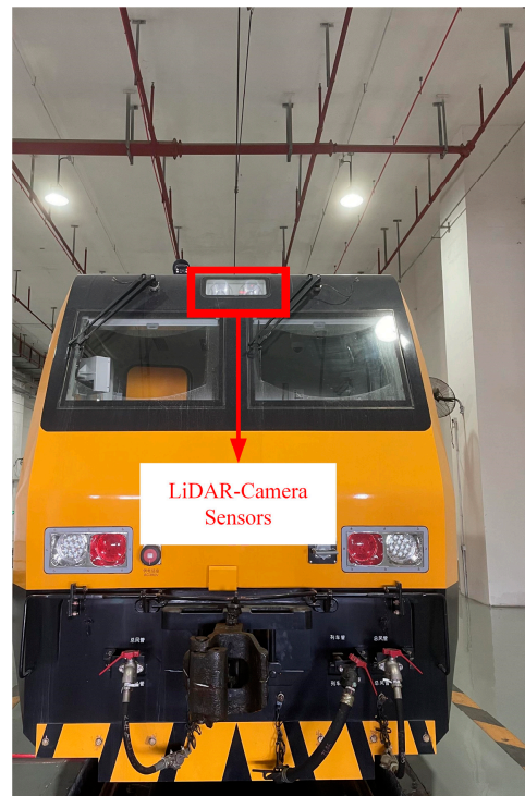
Figure 4. The LiDAR and camera are positioned at the top of the locomotive's front end, with their field of view centers parallel to the ground.
