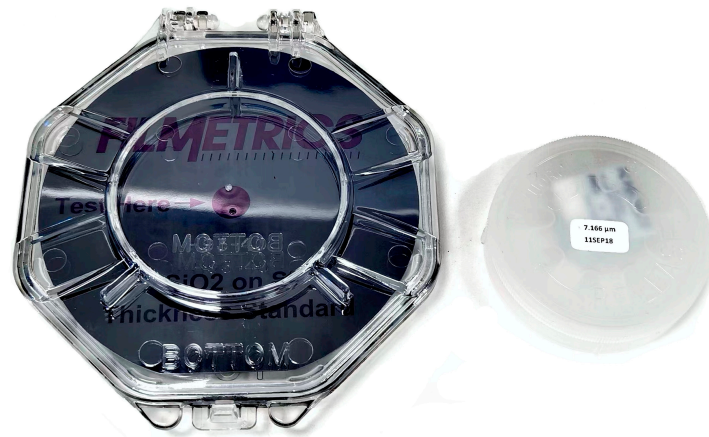
Figure 4. Photo of two standard film samples. Left: SiO 2 on Si thickness standard (Filmetrics, TS-SiO 2 -4-7200, San Diego, CA, USA). Right: parylene on Si thickness standard (Filmetrics, TS-Parylene-8um, San Diego, CA, USA).
