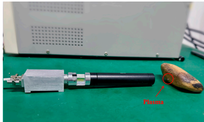
Figure 15. Laser excitation of microchip laser for the generation of plasma in stone.
