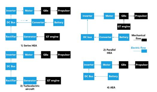
**Figure 1.** Simplified schematic of the propulsion system of EPA (adapted from [22]) (DC: direct current, GBx: power gearbox, and GT: gas turbine).
