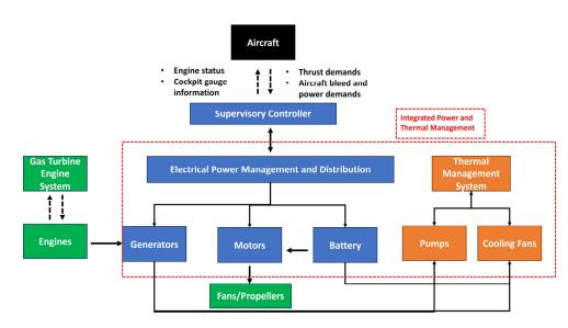
**Figure 2.** Control architecture for EPA, where the green blocks represent the engine system, blue blocks represent the power management system, and the orange blocks represent the thermal management system (adapted from [46]).
