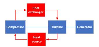
Figure 3. Simple IPTMS with energy recovery.
