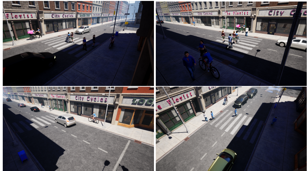
Figure 1. Exemplary images of realistic crowd simulation implemented in Unreal Engine. Such an approach gives an option for generating random pedestrian and car movement along with an option for including additional objects. It also enables the simulation of different light reflections and weather conditions.
