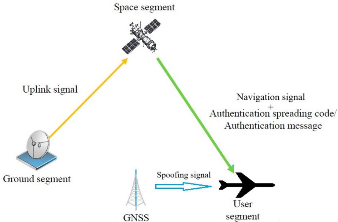
Figure 3. Satellite navigation system architecture with signal transmission. Prepared on the basis of [37].
