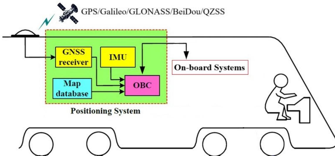
Figure 4. Example architecture of an on-board positioning system using a constellation of GPS/BDS satellites. Prepared on the basis of [28].
