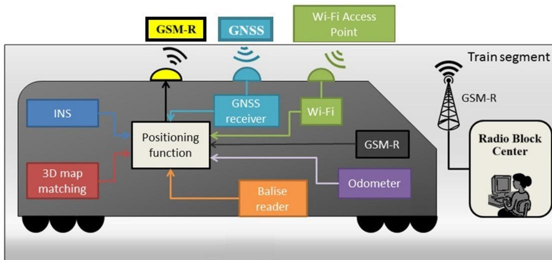
Figure 6. Physical architecture of a positioning system based on GNSS and Wi-Fi and GSM-R communications. Prepared on the basis of [63].
