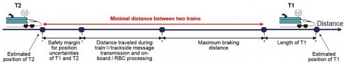
**Figure 12.** Principle of maintaining safe distances between train corridors. Prepared on the basis of [100].
