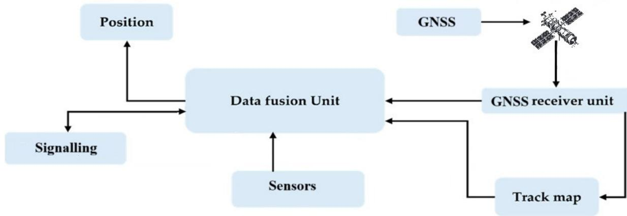
Figure 5. Basic architecture of a multi-sensor positioning system with GPS. Prepared on the basis of [46].
