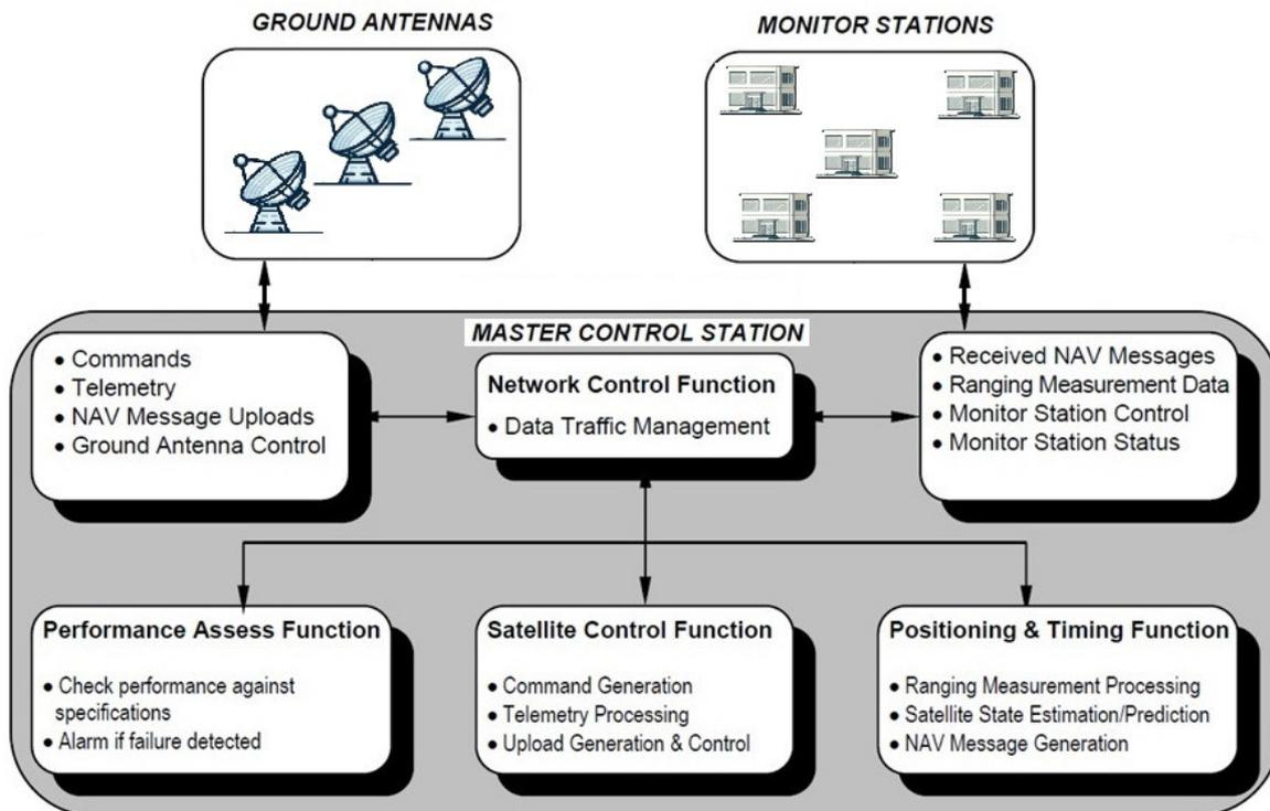
**Figure 8.** Ground (control) segment. Prepared on the basis of [69].
