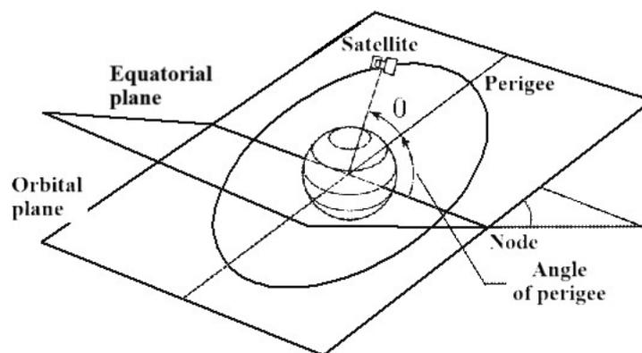
**Figure 7.** Orbital parameters of satellites. Prepared on the basis of [67].
