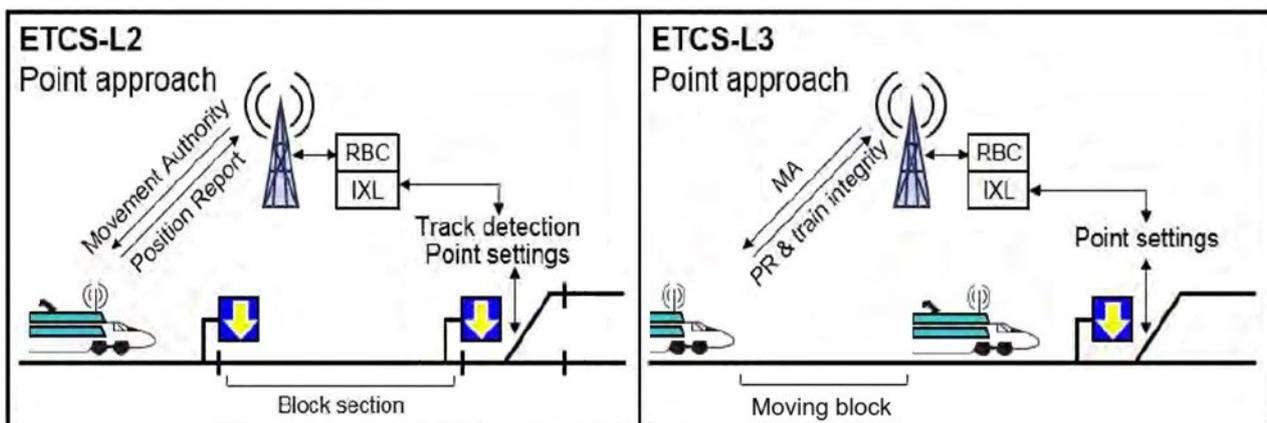
**Figure 11.** Functionality of the ETCS L2 and L3 system with respect to fixed and moving block spacing. Prepared on the basis of [100].
