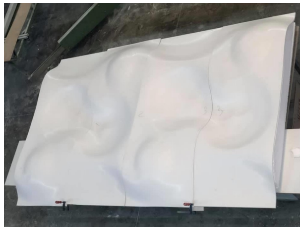
Figure 10. Assembly of 4 pieces of module B, composing the integrated modular part of the installed crawling area. Module A, not present, would attach to the left side.
