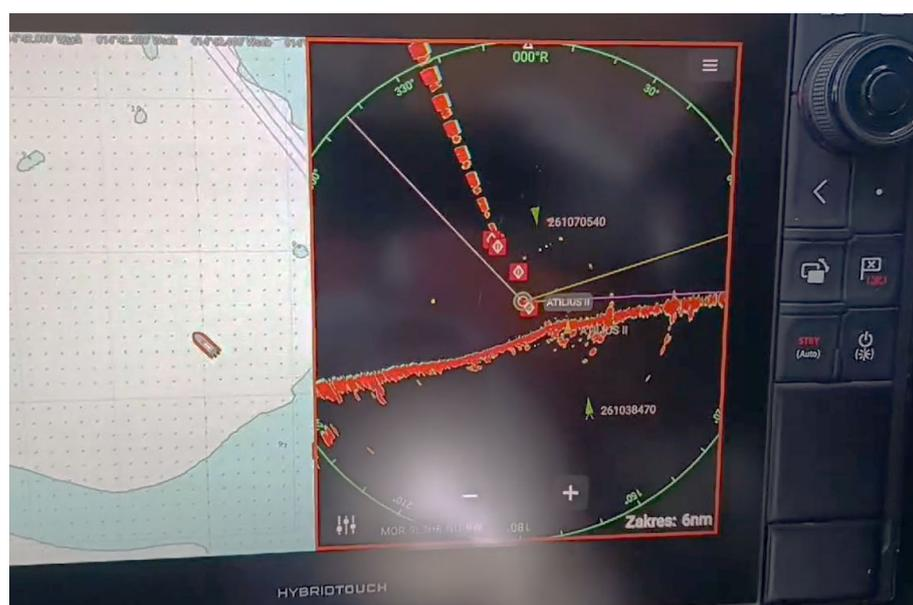
Figure 8. Radar screen showing the SART response signal at 2 Nm.
