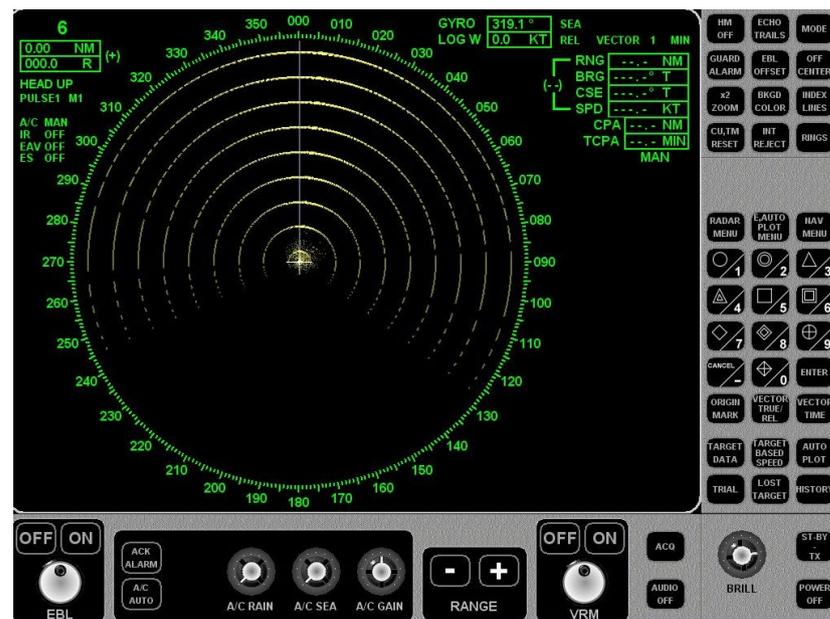
Figure 2. SART image on the radar [ECDIS Simulator NaviTrainer 5 Wartsila, Helsinki, Finland].
