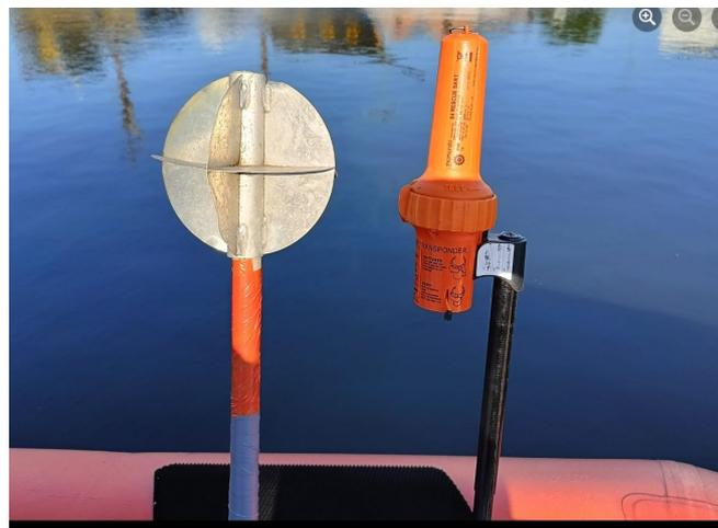
Figure 3. Radar reflector (left) and SART (right) placed next to each other on the liferaft.
