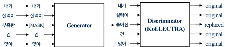
Figure 1. Structure and Operation of KoELECTRA’s Generator and Discriminator.
