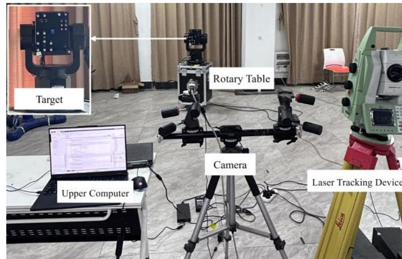
**Figure 11.** Experimental verification platform of attitude dynamic measurement system based on rotary table.
