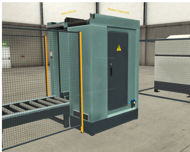
Figure 13. The danger zone of a machine (behind the door) protected by, among other things, an interlocking guard (own elaboration).
