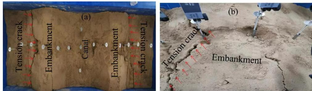
**Figure 8.** Tensile cracks. (a) Overall settlement of cracks in channel dykes; (b) canal crack.
