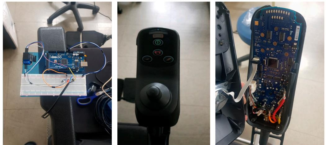
**Figure 9.** Hardware components and control interface of the motorized wheelchair system.
