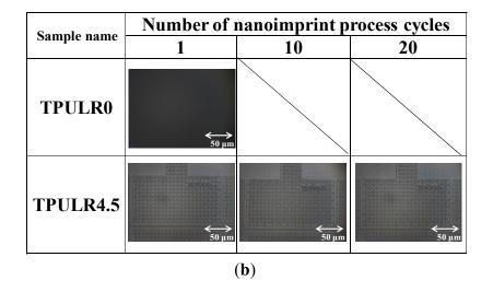
The resist patterns of the referenced TPULR0 without a UV reactive fluorine surfactant were non-imprinted after one imprint and almost part of the resist patterns was observed on the template. The template separation failure was considered to be due to the fact that the adhesion between TPULR0 and template was stronger compared with that between TPULR0 and the underlayer material TPU-UL, in the case of no approach to use a coated fluorinated self assembled monolayer on the surface of template.
