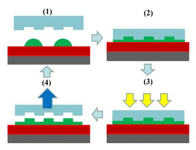
In order to obtain a better understanding of defect reduction on the template in nanoimprint patterning replication, the effect of an ultraviolet reactive fluorine surfactant, reacted with the main components in nanoimprint resist material, was evaluated using the above process cycles of UV curing nanoimprint lithography in this study.
