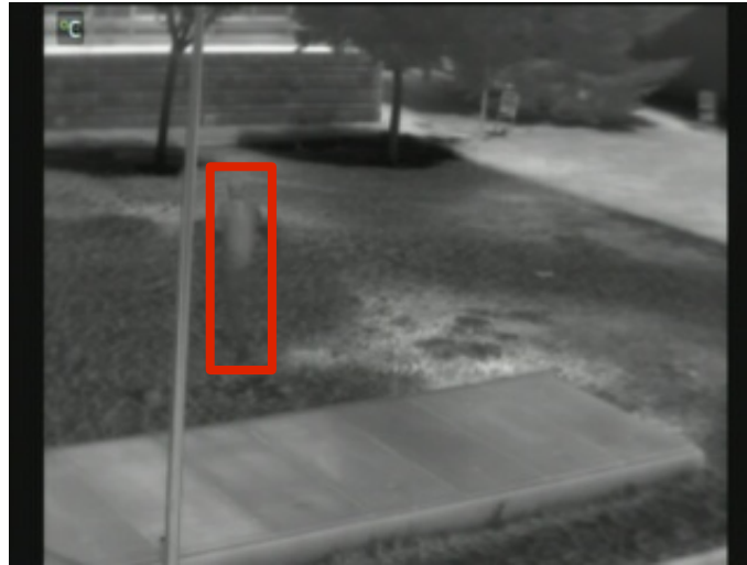
Figure 4. An example of a human being hard to detect in the thermal infrared spectrum.
