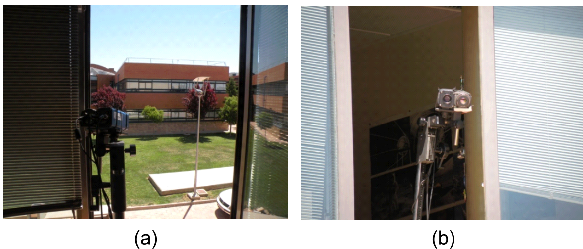
Figure 6. Installation for simultaneous acquisition on the thermal infrared and visible-light spectra. (a) Back view; (b) front view.
