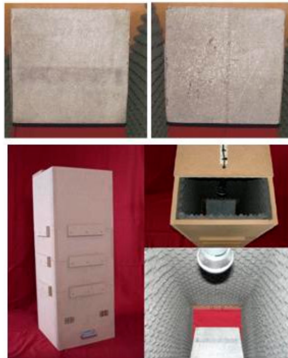
Figure 1. Stone plate for impact test and impact acoustic emission (AE) acquisition chamber.
