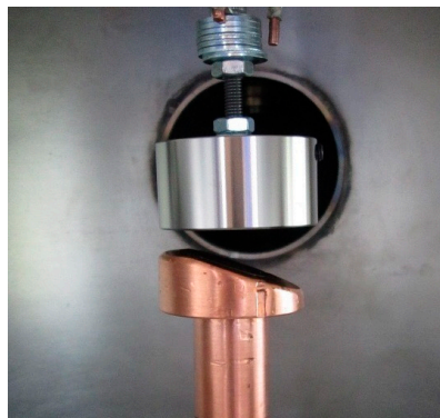
Figure 9. Photograph of the anode and cathode geometry in our X-ray tube; the anode material is Cu.
