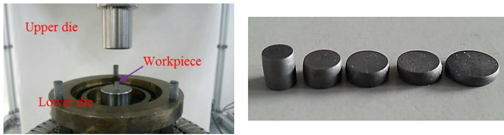
Figure 5. Compression experiment and compressed cylindrical samples at 30%, 60%, 75%, and 90%.
