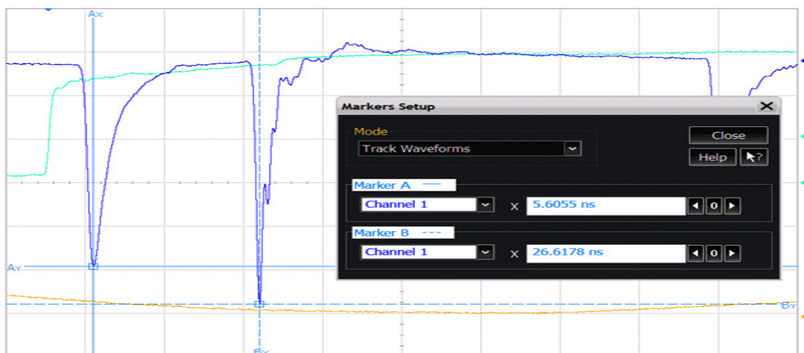
Figure 5. Signal waveforms measured by the Beam Current Transformers (BCTs).
