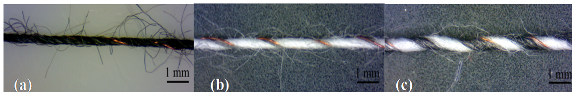
Figure 6. Stereomicroscopic observations of BC (a); PC (b) and BPC (c) ring-spun complex yarns.
