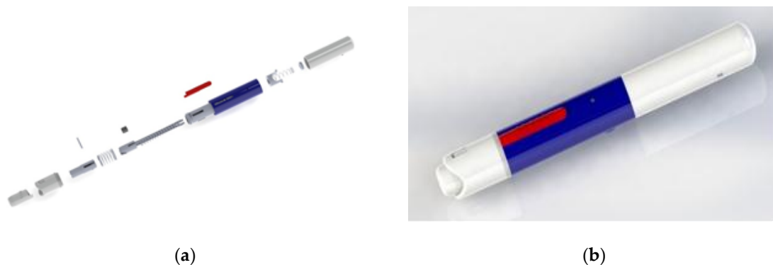
Figure 4. Innovative high-speed lancing device: (a) structurally expanded view; (b) schematic 3D assembly.
