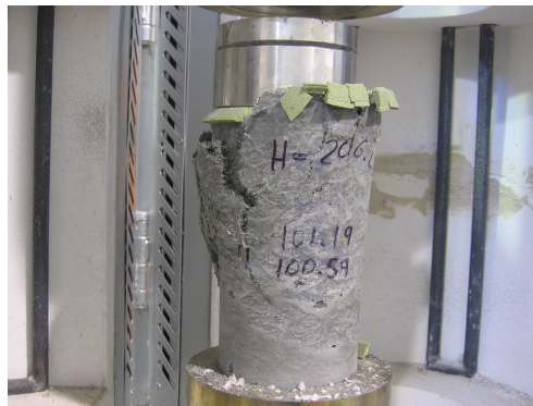
Figure 3. Destructive compression applied on an ECC specimen on Day-3.
