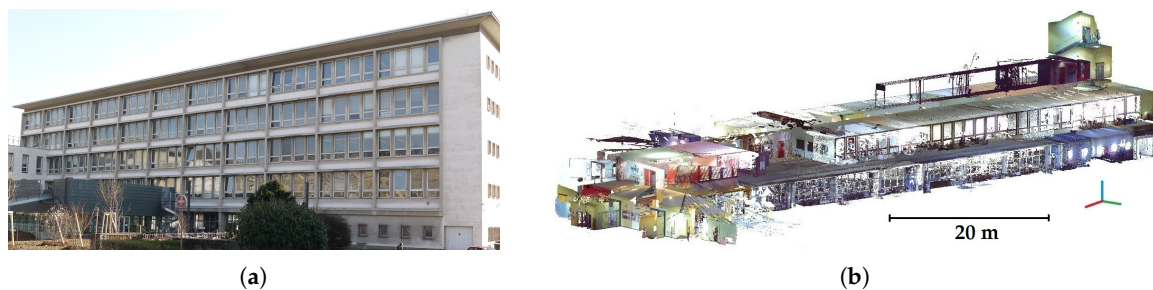
Figure 2. Dataset used to illustrate the approach: (a) Photograph of the acquired building. (b) Indoor colorized point clouds (~1.7 billion points before resampling).
