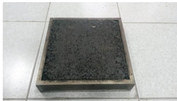
Figure 3. A square slab with dimension 305 \times 305 \times 50 mm.
