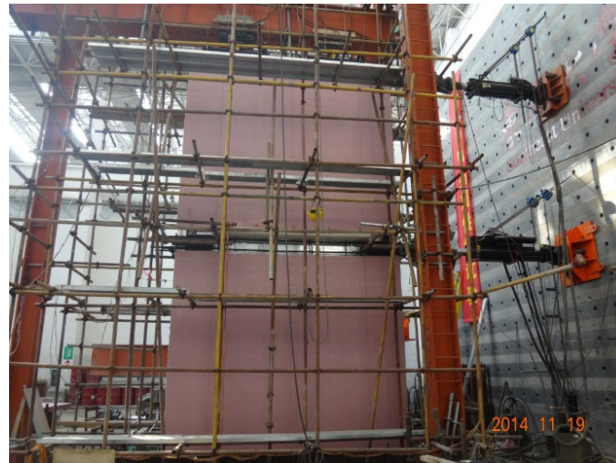
Figure 3. Cyclic loading tests of CFS shear wall systems.
