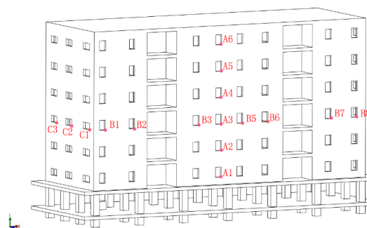
Figure 10. The location of the external monitoring points in six-layer model. A1–A6 are six monitoring points of vertical direction of the building; B1–B8 are eight monitoring points of horizontal direction of the building; C1–C3 are three monitoring points of the longitudinal direction of the building.
