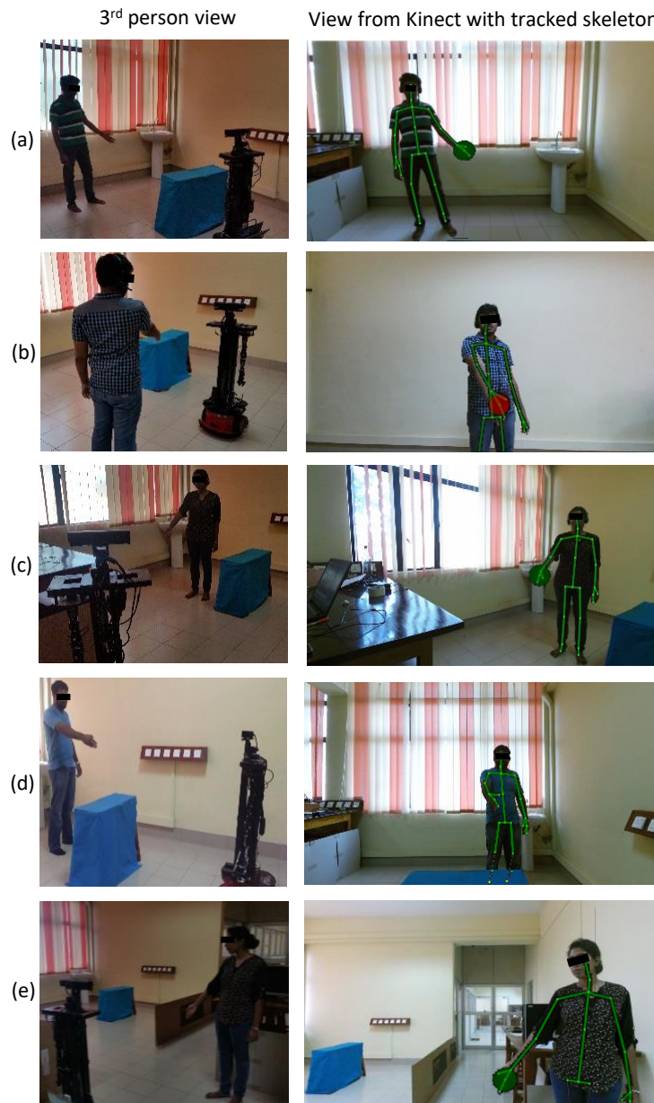
Figure 6. The view of the robot and the third person view of sample scenarios are shown with the corresponding case (a–e) given in Table 2. The tracked skeletons of the users are also superimposed with the RGB view of the robot for better clarity.
