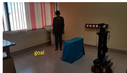
Figure 8. This shows the experimental scenario of the case 1 of the experiment for comparing the performance of the system with the MIS and the system without the MIS. The user was asked to navigate the robot to the goal position marked on the floor by implementing both the system in the robot. The goal area is annotated as “goal” in here.
