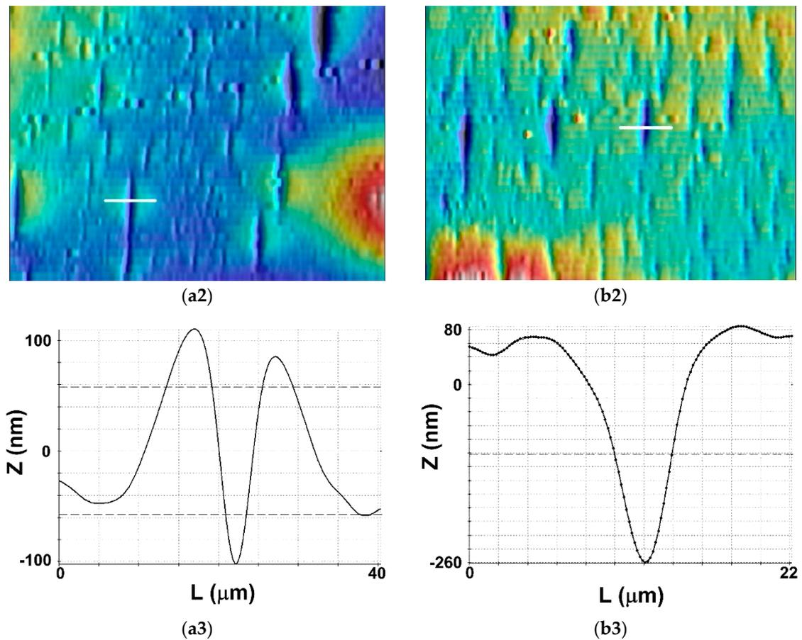
**Figure 18.** Typical surface morphology within necked area for samples programmed at 128 °C. Top row (1): 3D view; middle row (2): top view (area: 140 × 100 μm); bottom row (3) cross-section of the crack marked in middle row (2). Left: 30% strained; right: 100% strained.
