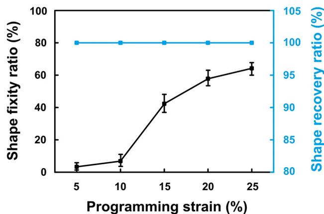
**Figure 7.** Shape fixity ratio and shape recovery ratio upon heating to 180 °C versus programming strain relationships for samples programmed at room temperature.
