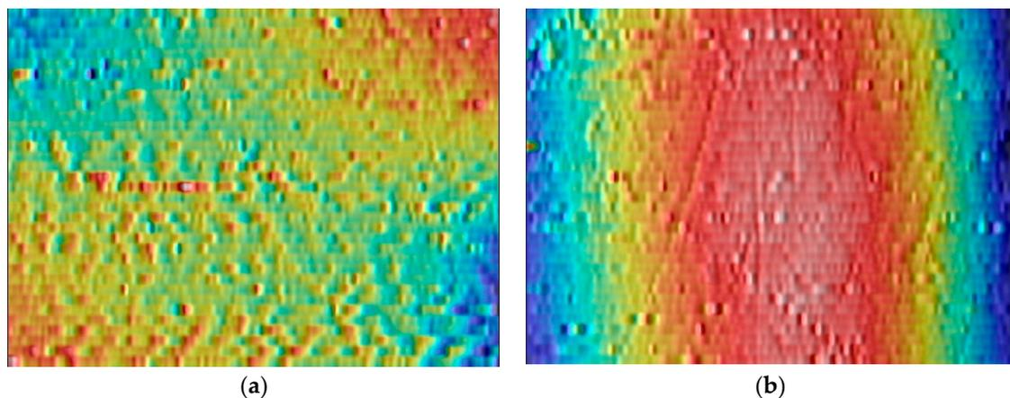
**Figure 19.** Typical surface morphology within non-necked area (140 × 100 μm). (a) 30% strained; (b) 100% strained.
