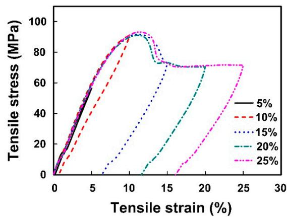
**Figure 6.** Typical stress versus strain relationships in uni-axial tension to five different programming strains at room temperature, and then followed by unloading.
