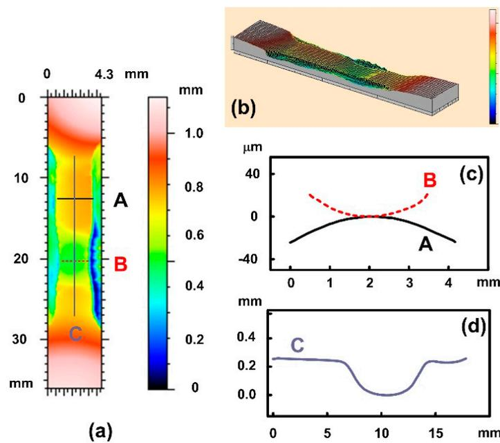
**Figure 13.** Surface morphology of sample programmed to 30% strain at 128 °C. (a) Top view; (b) 3D view; (c) surface profile of lines A (non-necked area) and B (necked area) as marked in (a); (d) profile of line C (throughout the gauge length of the sample) as marked in (a).
