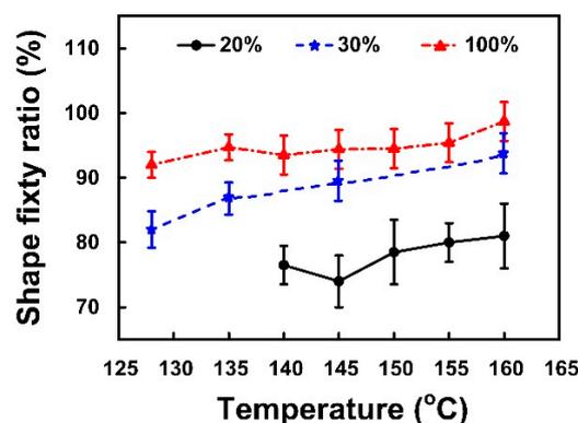
**Figure 9.** Shape fixity ratio ( $R_f$ ) against programming temperature with three different maximum programming strains.
