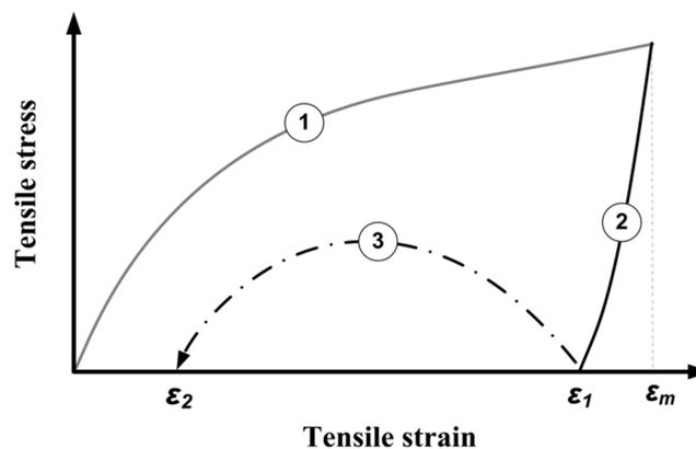
Figure 5. Illustration of stress versus strain relationship in a standard shape memory effect (SME) cycle. The numbers inside of the circles are meant for the steps.
