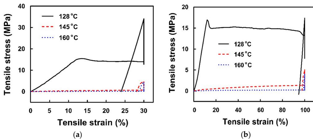
**Figure 8.** Typical stress versus strain curves in uni-axial tension at different temperatures to maximum programming strains of 30% (a) and 100% (b) and then unloading after cooling to room temperature.
