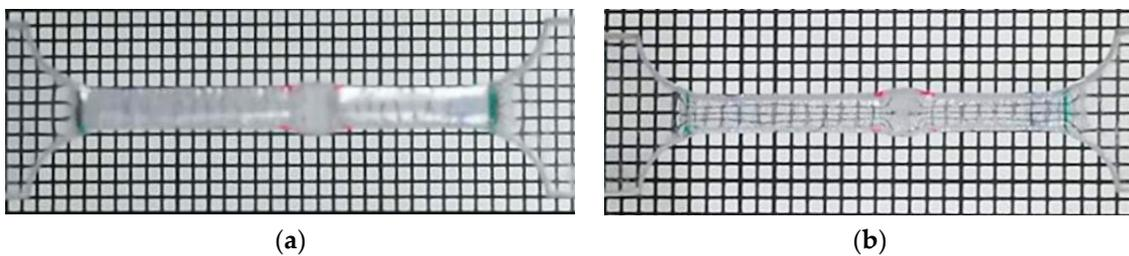
**Figure 16.** Lens effect in the sample programmed to 100% strain at 128 °C. (a) 56.5 mm above the grid paper (blur); (b) 13 mm above the grid paper (clear).
