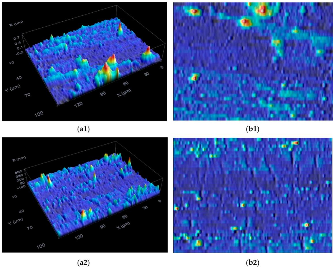
**Figure 20.** Typical surface morphology within the necked area in samples programmed at 135 °C. (a): 3D view; (b) top view. Top row (1): 30% strained; bottom row (2): 100% strained.
