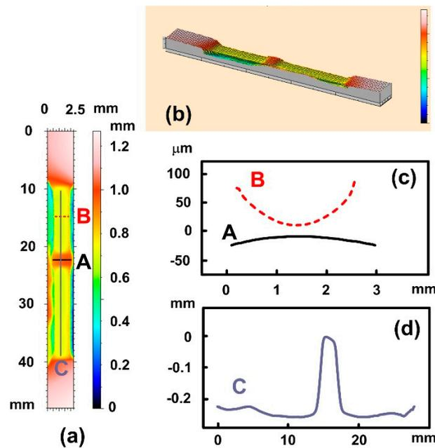
**Figure 14.** Surface morphology of sample programmed to 100% strain at 128 °C. (a) Top view; (b) 3D view; (c) cross-profile of lines A (non-necked area) and B (necked area) as marked in (a); (d) profile of line C (throughout the gauge length of the sample) as marked in (a).
