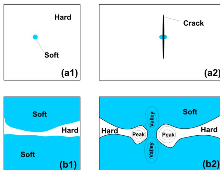
**Figure 22.** Formation of a short line crack (a) and a butterfly (b). Left (1): before stretching; right (2): after stretching.
