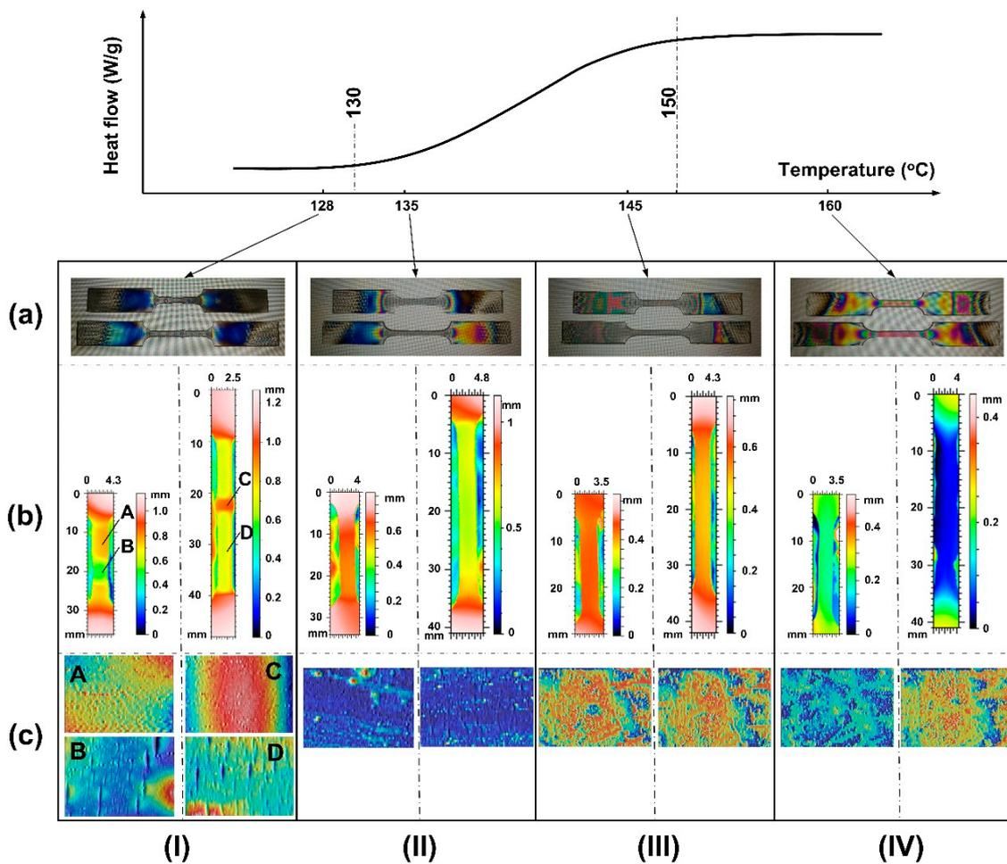
**Figure 11.** Summary of samples programmed to 30% and 100% strains at four temperatures of 128 °C (I); 135 °C (II); 145 °C (III) and 160 °C (IV). Top-subfigure: illustration of DSC curve. (a) Image of photo-elastic effect (top sample: 30% strain; bottom sample: 100% strain); (b) macro-scale 3D scanning result of sample surface (by Taylor Scanner); (c) micro-scale 3D scanning of zoom-in surface (area: 140 × 100 μm) (by PLμ Confocal Imaging Profiler).
