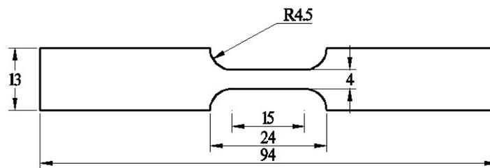
Figure 4. Dimensions of dog-bone shaped sample (according to ASTM D638, Type IV).
