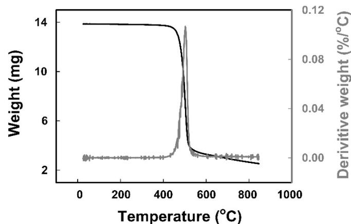
**Figure 2.** Typical thermogravimetric analysis (TGA) result. Black line: weight; grey line: derivative weight.
