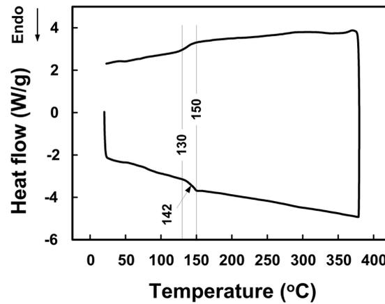
Figure 3. Typical differential scanning calorimetric (DSC) result (the second cycle).
