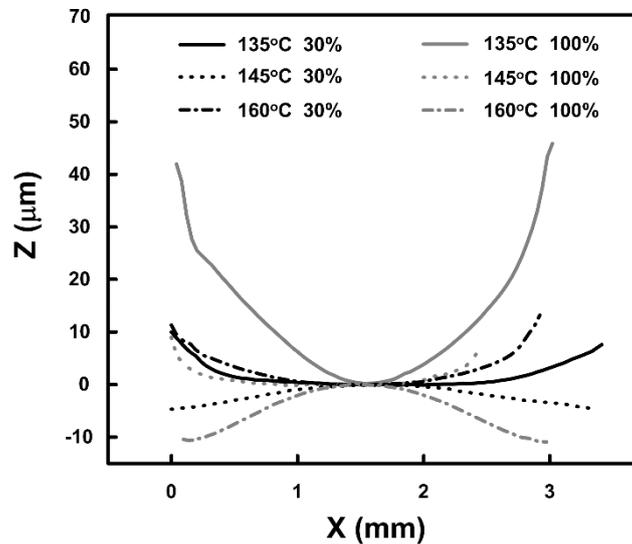
Figure 17. Comparison of typical cross-sections in samples programmed at 135 °C and above.
