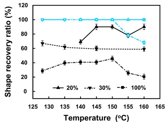
**Figure 10.** Shape recovery ratio ( $R_r$ ) as a function of the programming temperature and programming strain. Black line: upon heating to the programming temperature; blue line: upon further heating to 180 °C.
