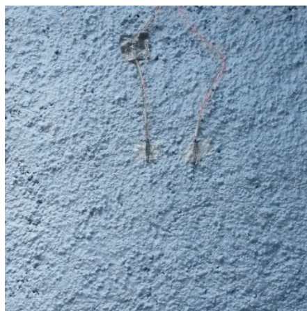
Figure 1. The phase change material (PCM)-perlite composite placed on mineral wool insulation component.
