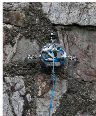
Figure 15. Stably grabbing the granite wall.
