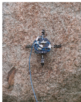
Figure 16. Stably grabbing the rough rock wall.
