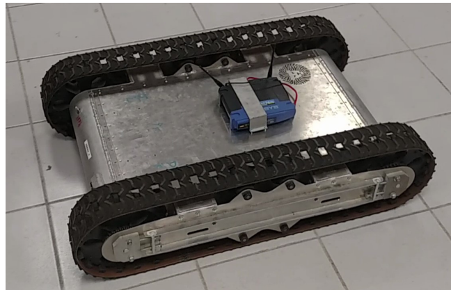
Figure 3. Modified HD2 ® Treaded All-Terrain Tracked Robot (ATR) Tank Robot Platform with wireless communication.
