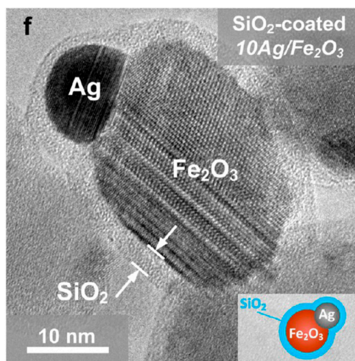
Figure 7. HR-TEM image of silica coated \text{Ag-Fe}_2\text{O}_3 dumbbell synthesised by flame spray pyrolysis. Reprinted with permission from [56]. Copyright ACS, 2013.
