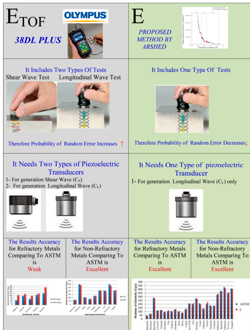
Figure 10. Comparison between time-of-flight (TOF) method and Arshed method.
