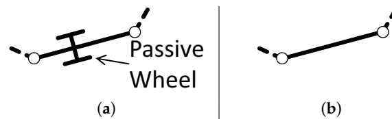
Figure 1. The distinction between a side-slipping link and a non side-slipping link. (a): a non side-slipping link. (b): a side-slipping link.
