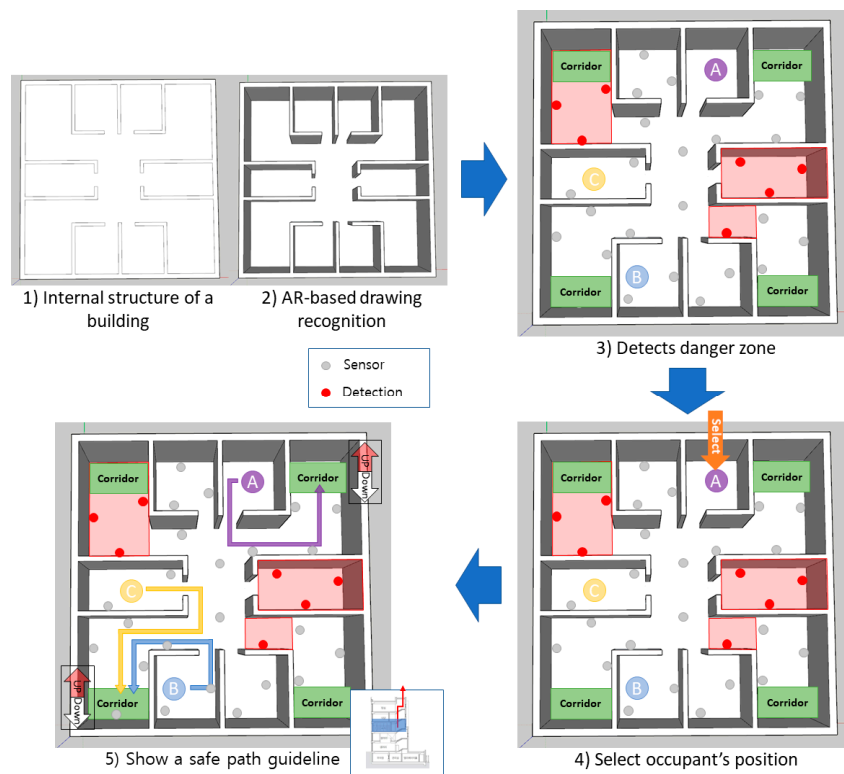
Figure 17. System operation for occupants.
