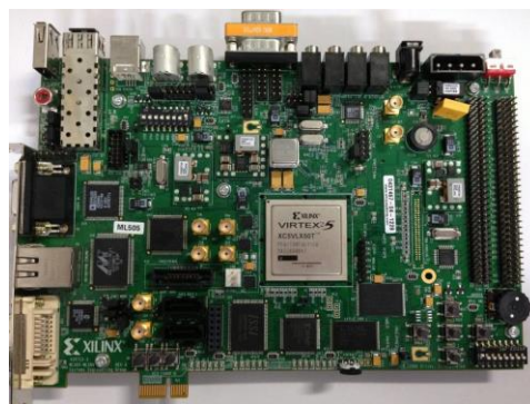
Figure 12. Xilinx ML505 field-programmable gate array (FPGA) evaluation board.
