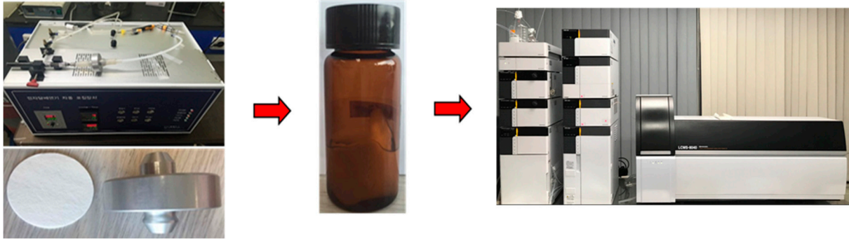
(a) Type 1: Sampling the aerosol using Cambridge filter pad (CFP)
